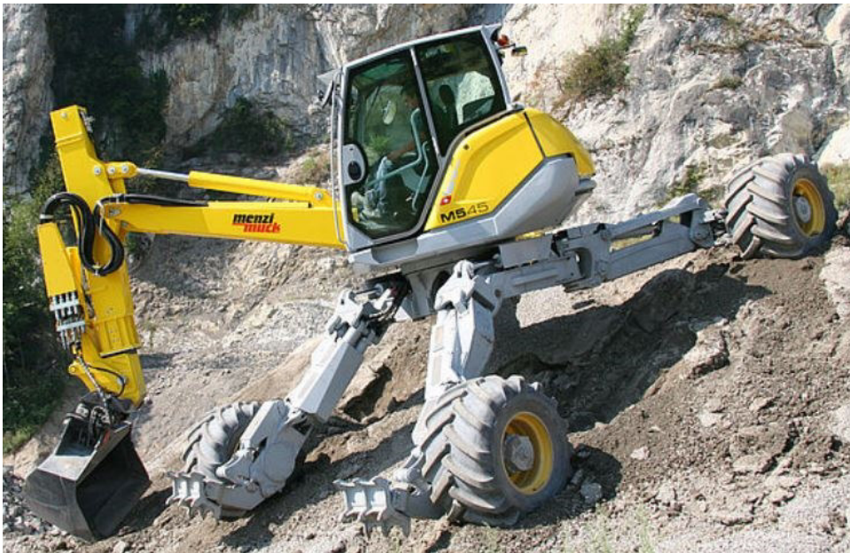
Figure 2.1: Menzi Muck's walking excavator M545; Source: [1]
