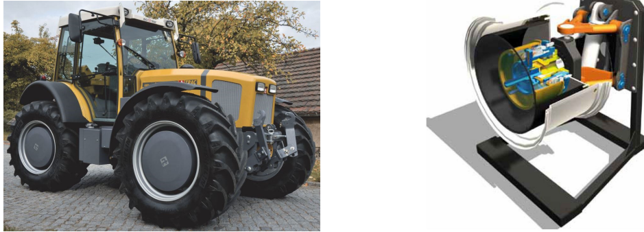
Figure 3.5: Picture of the Rigitrac EWD 120 (Source: [10]) and scheme of the corresponding electric wheel hub drive (Source: [11])
