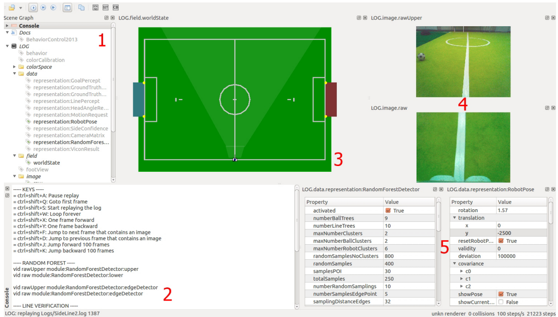
Figure 2.2: Example screenshot of the SimRobot user interface: (1) Scene Graph to select required data; (2) Console for commands; (3) WorldState to track positions of objects on the soccer field; (4) Images of robot’s upper and lower camera; (5) Data of representations
