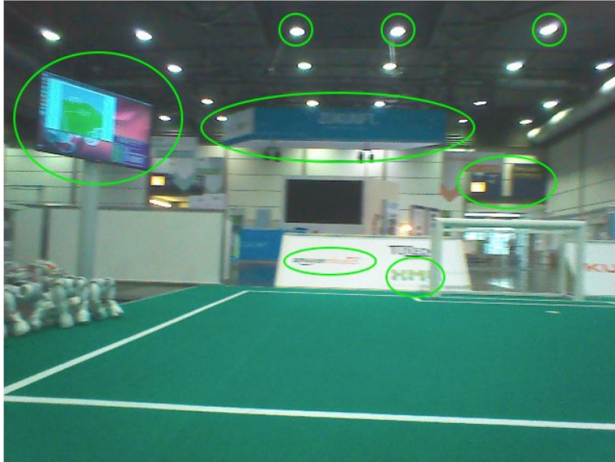
Figure 5.2: Examples for external features at a RoboCup tournament which can be used to find a prior robot pose; Source: [16]
